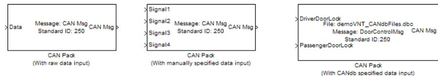
The CAN Pack block loads signal data into a message at specified intervals during the simulation.
