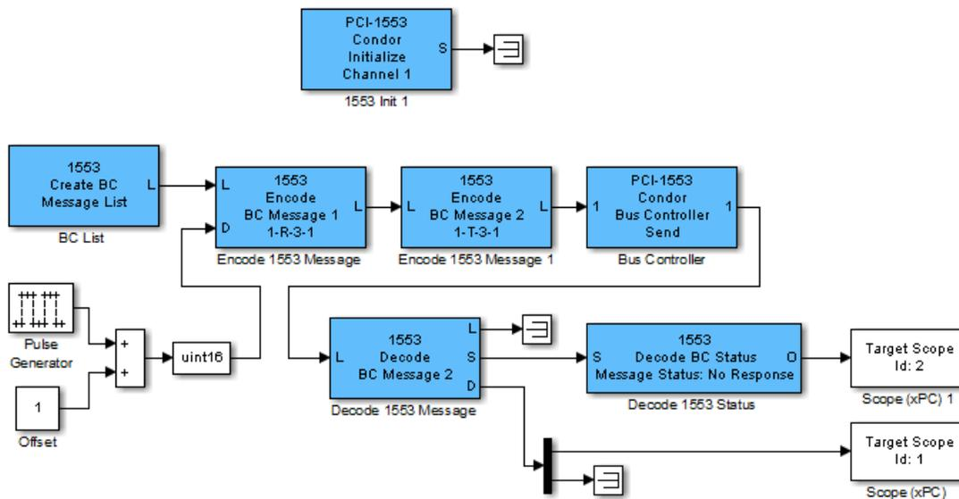
The PCI-1553 Initialize block configures a Bus Controller on channel 1 of the board. This block also tells the board to reserve five message buffers. This number must be at least as large as the longest list of messages that you will send.
