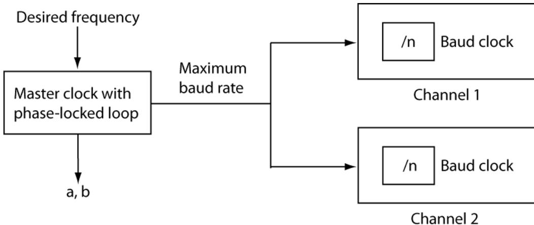
To set the block parameters for this board, choose a maximum baud rate, as follows. This procedure assumes that both channels require different baud rates. Determine a common base clock that can be divided to produce the required baud rates for both channels, as follows:
