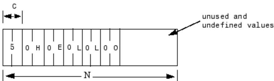
These serial blocks interpret each entry in the vector as a single character. The low-level Send block writes the low-order byte of each entry to the UART. The 16- and 32-bit data types allow the embedding of 8-bit data values, including 0. The 8-bit data type is most useful with the ASCII Encode and Decode blocks. The 16- and 32-bit data types are most useful for binary data streams.
