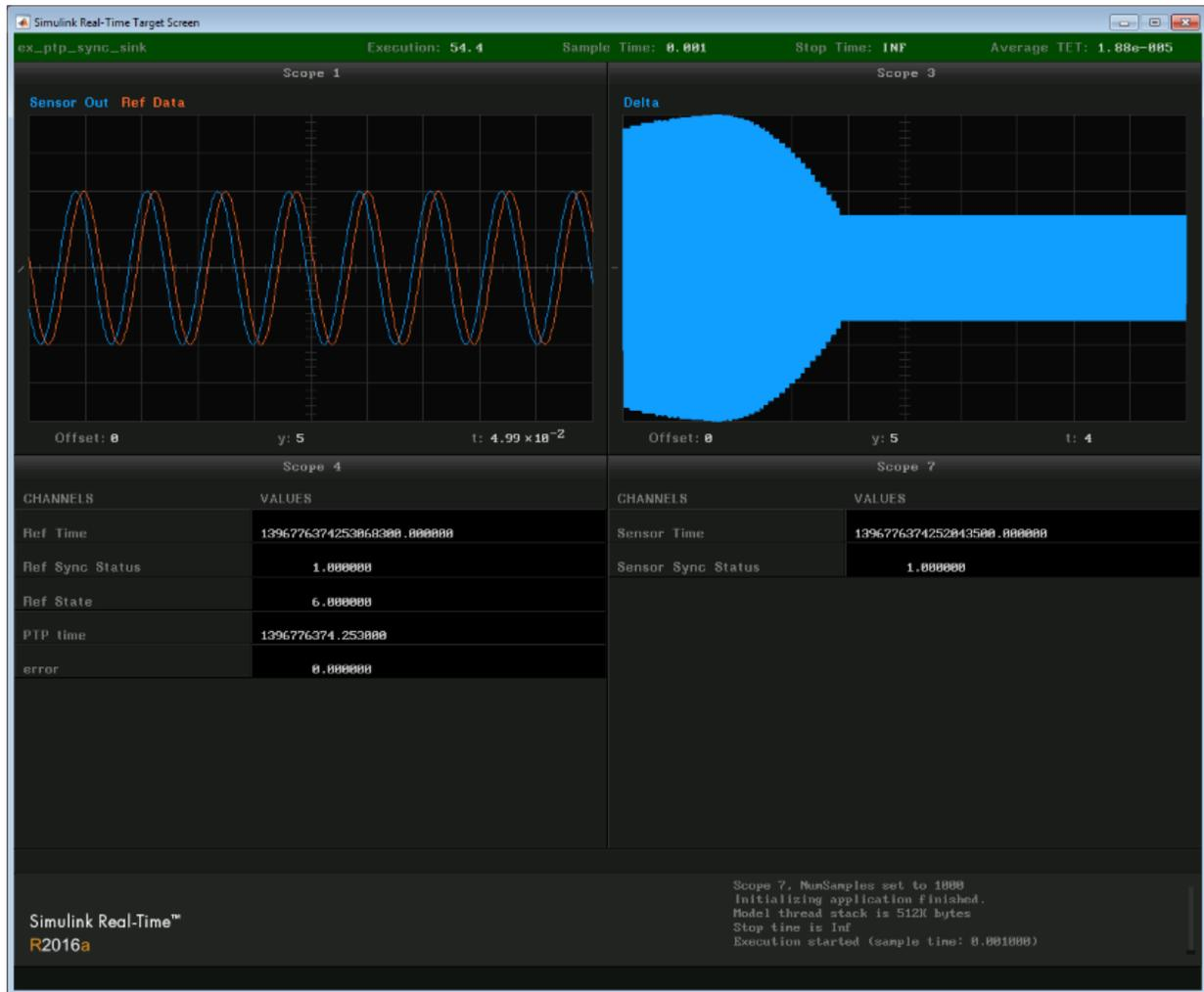
For this example, the sensor and reference Sine Wave blocks are set to the same frequency and amplitude, but start at arbitrary times. The difference in start time causes a phase difference between the sine waves. The phase difference appears on the Delta scope as a waveform that settles to a constant amplitude.
