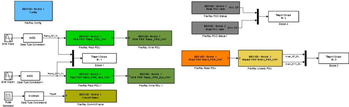
Invert\_ECU: Reads PDU received from Ramp\_ECU and sends back the received signals to Ramp\_ECU.
