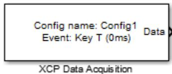
The XCP Data Acquisition block acquires data from the configured slave based on the selected measurements. The block uses the XCP CAN transport layer to obtain raw data for the selected measurements at the specified simulation time step. Configure your XCP connection and use the XCP Data Acquisition block to select your event and measurements for the configured slave. The block displays the selected measurements as output ports.
