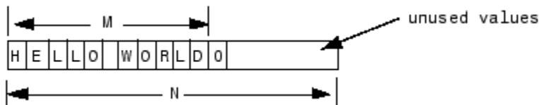
This string has 11 characters terminated with a NULL byte (0). This data type cannot contain a NULL byte as part of the real data.
