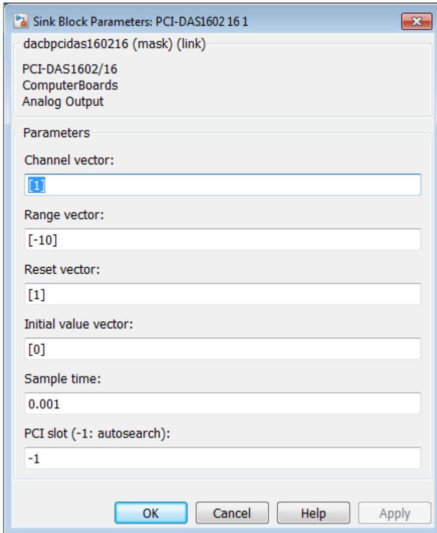
If you change the sample time by changing the target object property `SampleTime`, the sample times you entered in both of the I/O blocks are set to the new value. The step size you entered in the Configuration Parameters dialog box remains unchanged.
