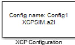
The XCP Configuration block uses the parameters specified in the A2L file and the ASAP2 database to establish XCP slave connection.
