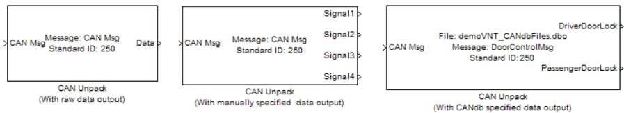
The CAN Unpack block unpacks a CAN message into signal data using the specified output parameters at every timestep. Data is output as individual signals.
