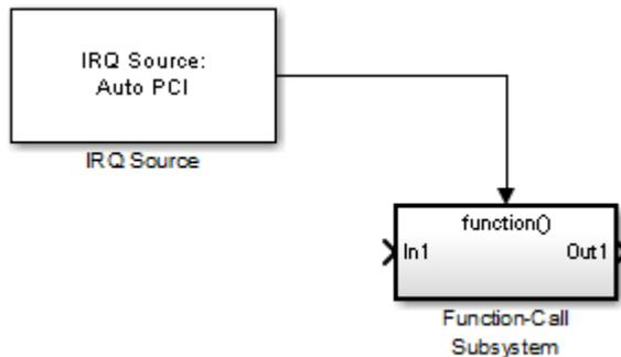
In the setup shown above, the CPU executes the contents of the Function Call-Subsystem whenever IRQ 5 occurs.
