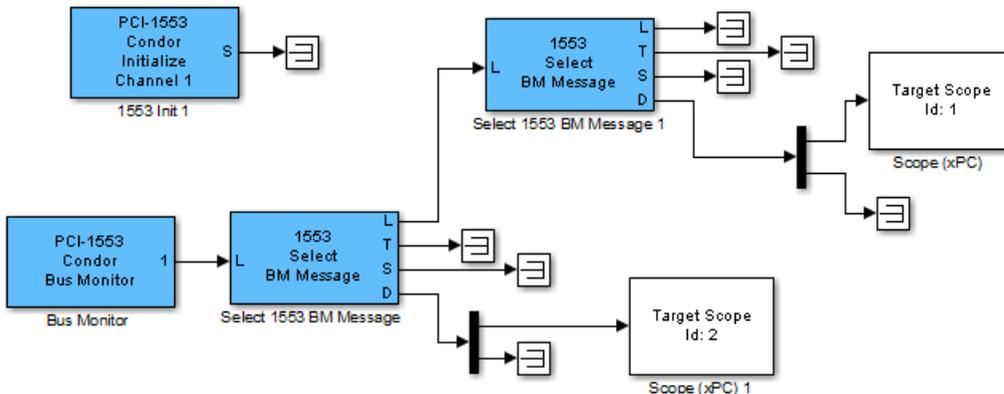
The PCI-1553 Initialize block configures a Bus Monitor on channel 1 of the board. This block also instructs the board to monitor bus A.
