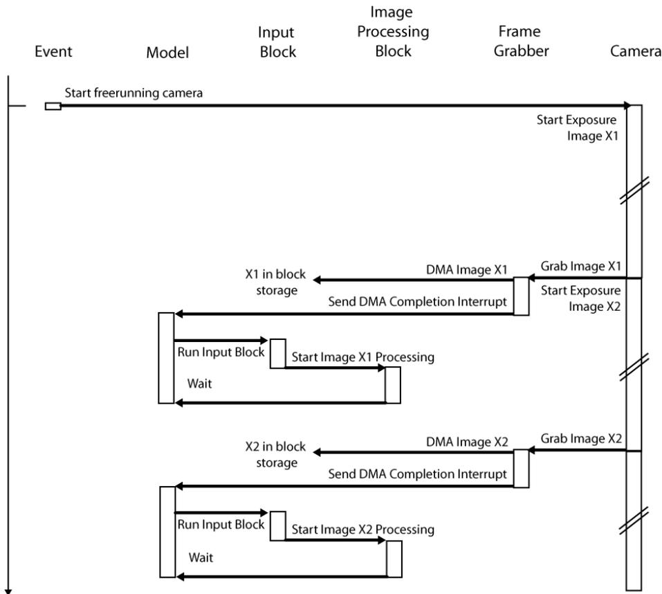
Before the next DMA completion interrupt, the model must complete image processing. Otherwise, the CPU becomes overloaded.
