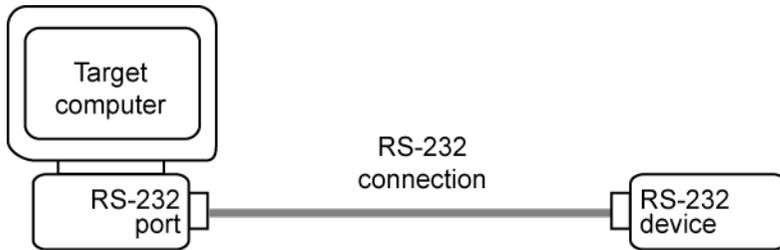
Your real-time applications can use these RS-232 ports as I/O devices. With the typical DTE/DCE configuration of the RS-232 device, the target computer is connected to the device with a null modem cable.
