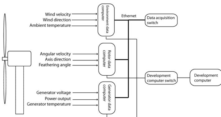
To record the data and timestamps, you connect the sensors to a set of data acquisition target computers. You interconnect the data acquisition computers through an Ethernet network and a switch that supports the PTP protocol (a PTP transparent clock or boundary clock). To access the data and timestamps, you connect the target computers
