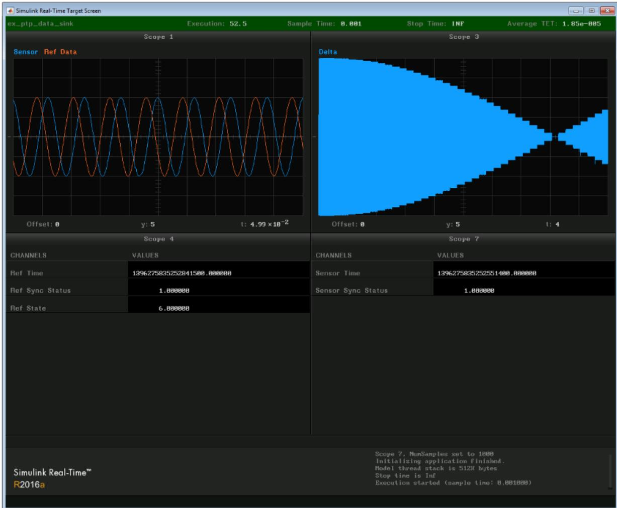
With the IEEE 1588 Sync Execution block, you can make measurements across multiple target computers at a synchronized time step. However, the kernel interrupt clock
