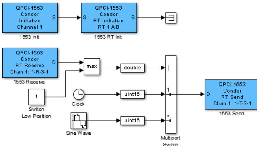
The QPCI-1553 Initialize block configures the board for Remote Terminal operation on channel 1 of the board. The QPCI-1553 RT Initialize block configures the Remote Terminal 1 to monitor buses A and B for incoming messages and configure the active transmit and receive sub addresses. The QPCI-1553 Receive and Send blocks use sub address 3 for both transmit and receive. Note the message parameters notation 1-R-3-1 on the QPCI-1553 Receive and Send blocks. This notation has the format:
