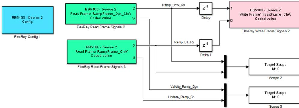
Before configuring model `dFlexRaySimpleExample_ErrorInjection`, record the bus and slot numbers of the FlexRay boards in the target computer and configure each FlexRay node.
