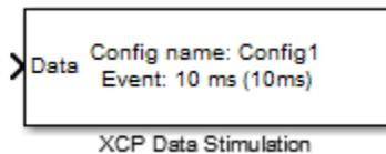
The XCP Data Stimulation block sends data to the selected slave for the selected event measurements. The block uses the XCP CAN transport layer to output raw data for the selected measurements at the specified stimulation time step. Configure your XCP session and use the XCP Data Stimulation block to select your event and measurements on the configured slave. The block displays the selected measurements as input ports.
