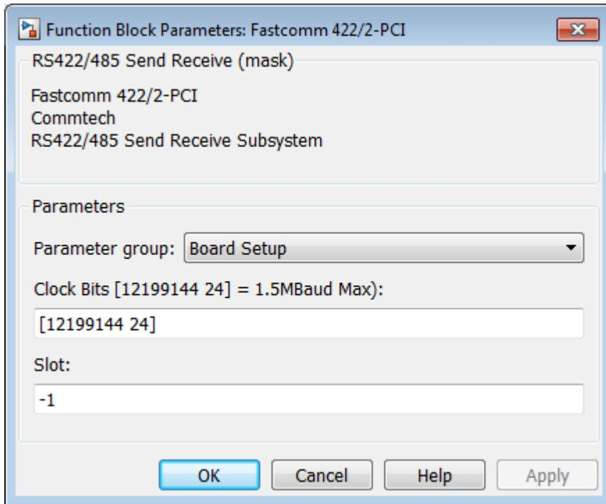
After you define a maximum baud rate, you can set a unique baud rate for each channel by choosing a different baud rate divisor for each channel. For example, you can have Channel 1 have a baud rate of 750000 (1500000/2) and Channel 2 have a baud rate of 1500000 (1500000/1). To set Channel 1 to have a baud rate of 750000, with the Fastcom 422/2-PCI Send Receive block with the **Parameter group** parameter set to **Basic Setup**, set
